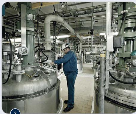
Facilities for downstream processing (reaction vessels in the foreground)
